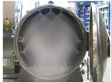
The system combines the steam-air mixture with superheated water spray, which is circulated at high speed by a pump through multiple spreaders over the top and at each side of the packages
